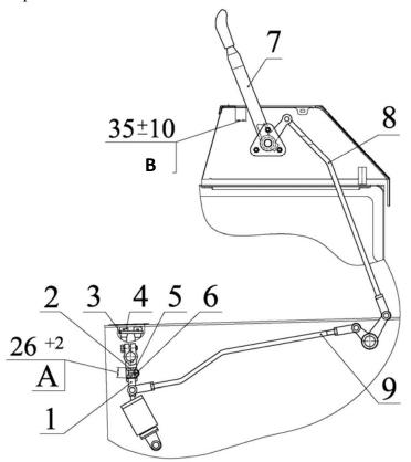
1 - lever; 2, - bolt; 3 - stopping device; 4 - adjusting screw; 5 - nut; 6 - service bolt; 7 - PTO engagement lever; 8 - link; 9 - link.
