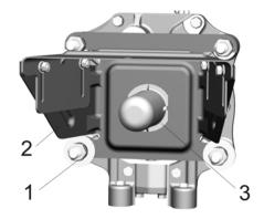
Figure 1a – Disassembly of PTO shaft end extension cap safeguard 1 - nut; 2 - safeguard; 3 - cap.
